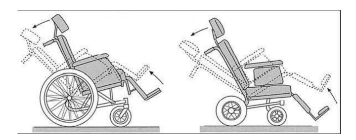
Small front wheels make the wheelchair mechanism lighter.
